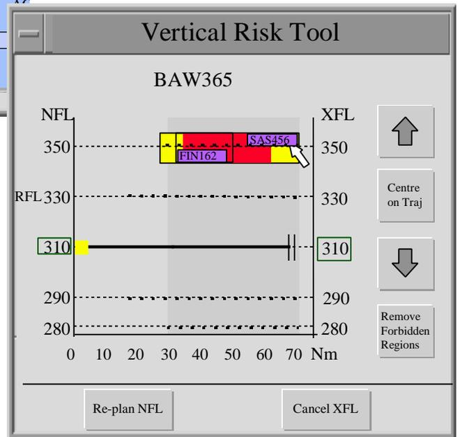
The tactical controller's VRT is similar to the planner controller's except that it only shows the trajectory for 10 minutes ahead and there are no buttons to support coordination.
