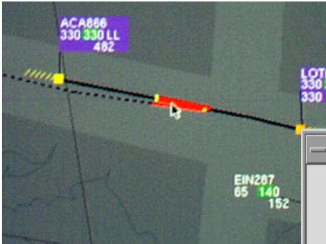
The LRT appears on the situation display when a controller “hooks” an aircraft by clicking on the callsign with the computer mouse, showing the trajectory of the hooked aircraft and any conflicts predicted along it. The trajectories of the conflicting aircraft are also shown. Conflicts are shown as coloured regions of the trajectory, red indicates an unacceptable conflict whilst yellow indicates an uncertain conflict. An example of the LRT is shown in the figure above.
