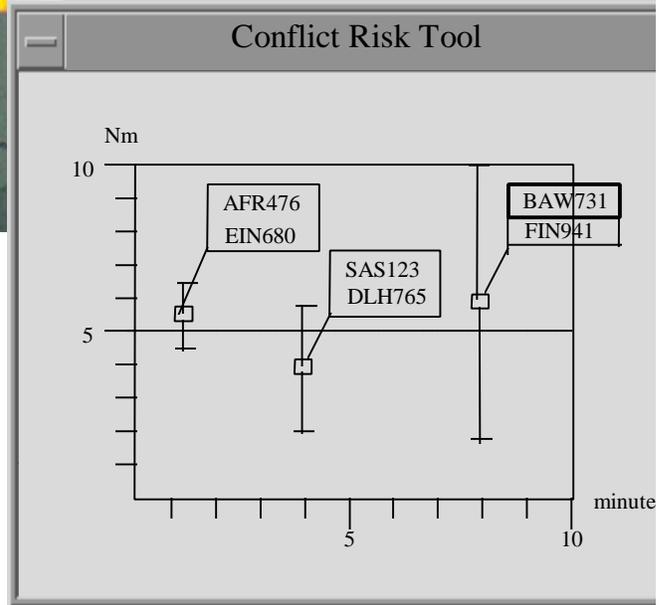
The uncertainty associated with the predictions is shown by the length of the vertical bars attached to each box. The callsigns of the aircraft concerned are also shown.
