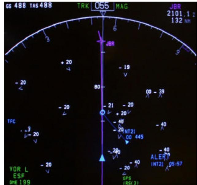
Figure 1. CDTI-AL on the flight deck navigation display.
