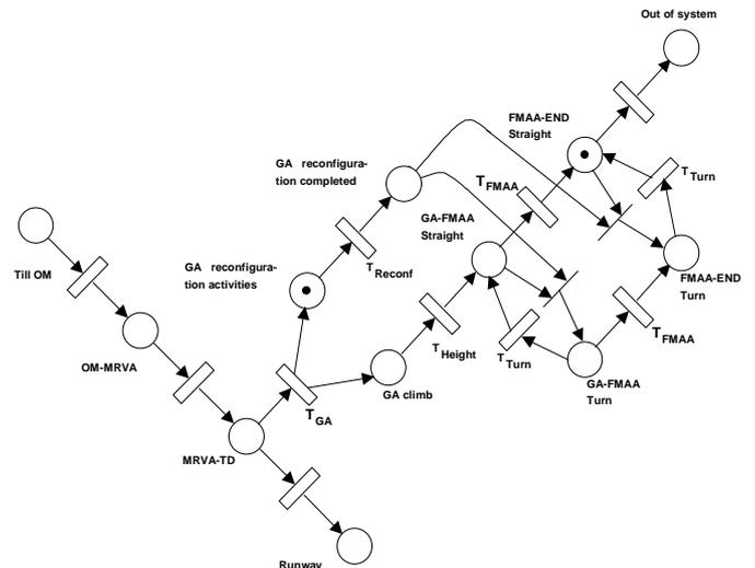
Figure 4 Aircraft evolution Petri net: detailed level. Drawn is a feasible two token situation, one token in place 'GA reconfiguration activities' and one token in place 'FMAA-END Straight'. Then the immediate transition to 'FMAA-END Turn' will fire as soon as the guard function of  $T_{Reconf}$  evaluates to true.
