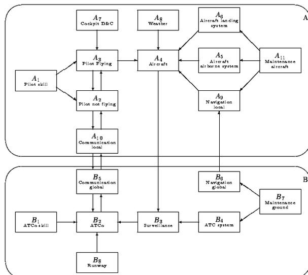
Figure 3 Functional representation of ATM.
