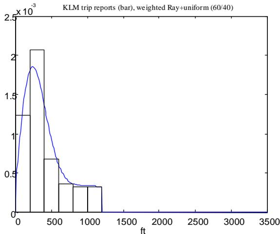
Figure 2 Histogram of KLM pilot GA trip reports and of density fit which is a weighted sum of a Rayleigh density (60%) with mean 300ft and a Uniform density on 0-1200ft (40%).
