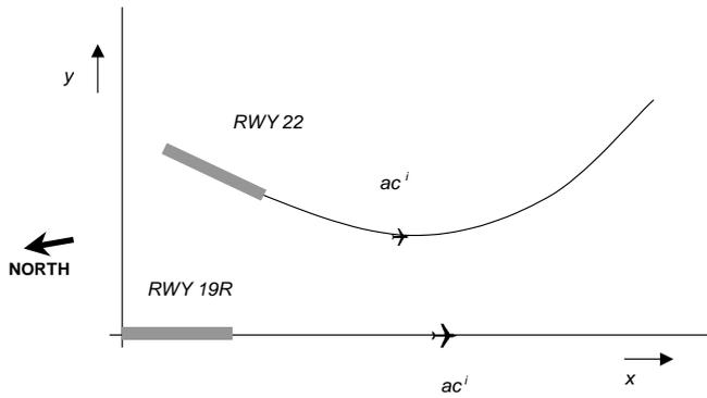
Figure 1 Geometry of runways 19R and 22 at Schiphol airport and the nominally performed missed approach paths.
