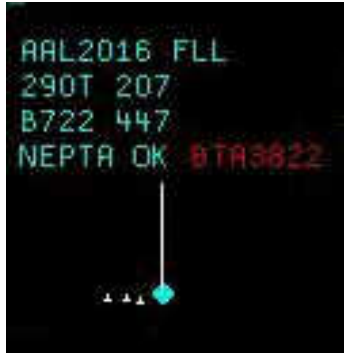
Fig. 2. Flight Data Block with direct route advisory and conflict information.
