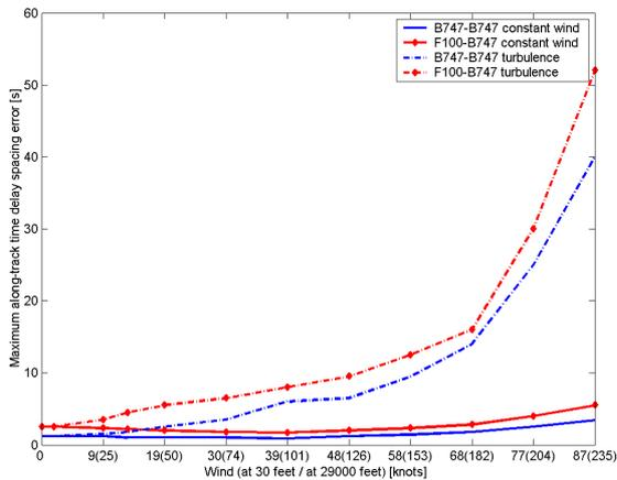
Figure 6. Tail wind effects on CTD spacing
