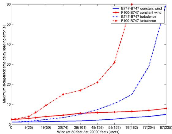
Figure 8. Cross wind effects on CTD spacing
