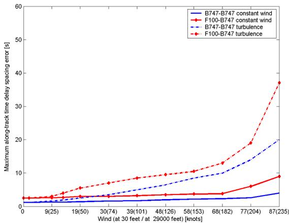
Figure 7. Head wind effects on CTD spacing
