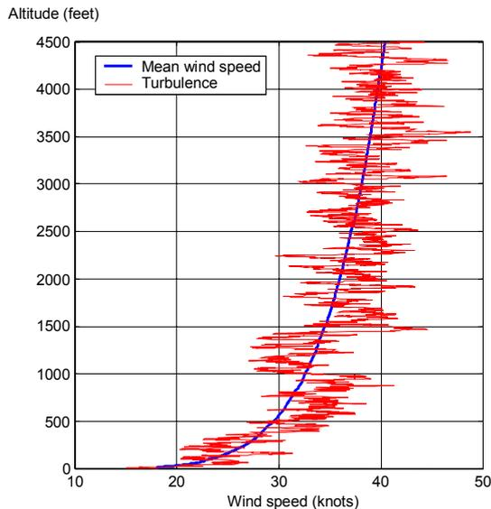
**Figure 2. Turbulent wind versus altitude - JAR-AWO model (20 knot wind at 30 feet)**
