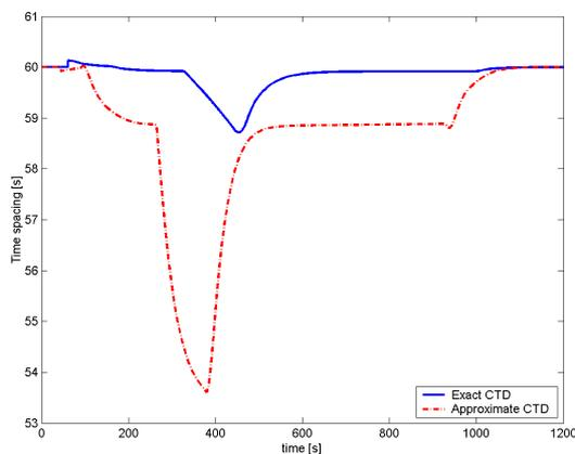
**Figure 5. Approximate and exact CTD criteria - time spacing**
