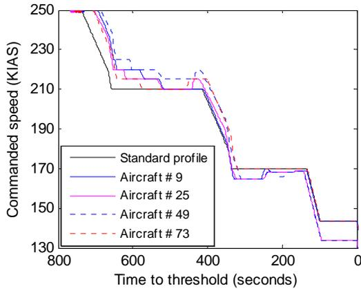
**Figure 5. Speed Profiles In A Nominal Scenario**
