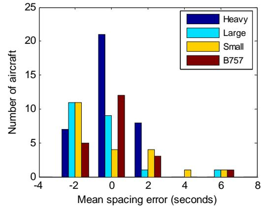
**Figure 12. Histogram Of Spacing Errors In Nominal Test Condition, Averaged By Aircraft Category**
