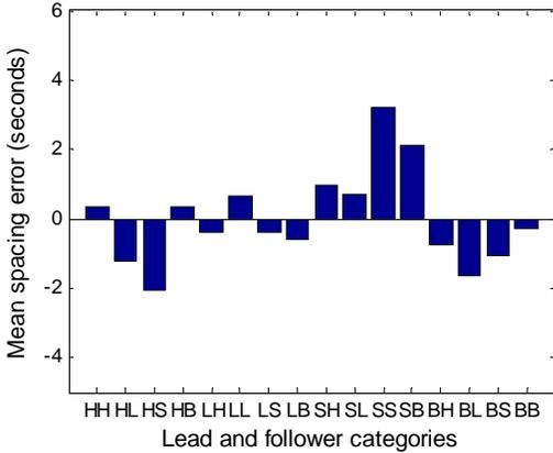
**Figure 13. Spacing Errors In Nominal Test Condition, Averaged By Lead And Follower Aircraft Categories (Nomenclature: H = Heavy, L = Large, B = B757, S = Small, HL = Heavy aircraft leading a Large aircraft, etc.)**
