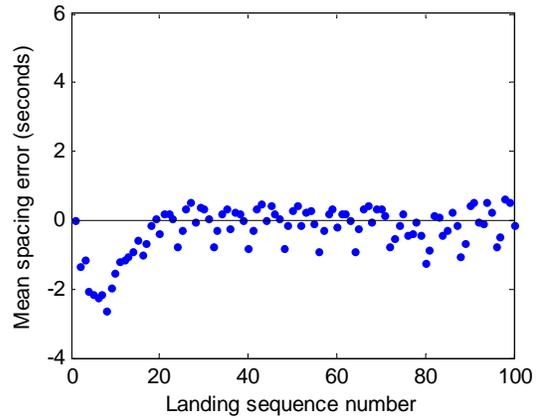
**Figure 14. Mean Spacing Errors For Homogenous Arrival Stream**
