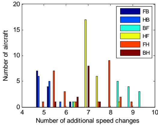
**Figure 17. Histogram Of Mean Number Of Additional Speed Changes For Homogenous Stream, Grouped By Entry Fix Combination (Nomenclature: F = FEVER, B = BAMBE, H = HOWDY, FB = Aircraft from FEVER leading aircraft from BAMBE, etc.)**
