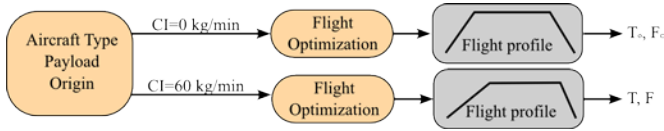
Figure 5: Schema of the flight optimizations performed for each flight in the data set
