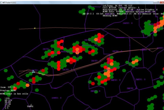
Figure 4. Probe flights on parallel tracks traversing ZKC in west-east direction when more weather is considered non-permeable. All flights have to be rerouted and the majority have to be delayed as well. There is only one lane available to traffic in this west-east direction.
